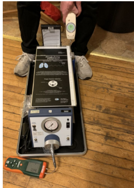
Figure 5. An image showing how the maximum required force was found
