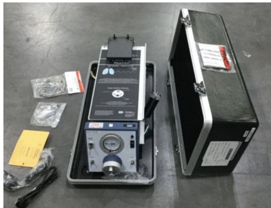
Figure 1. An image of the Michigan Instruments Test Lung with its case
