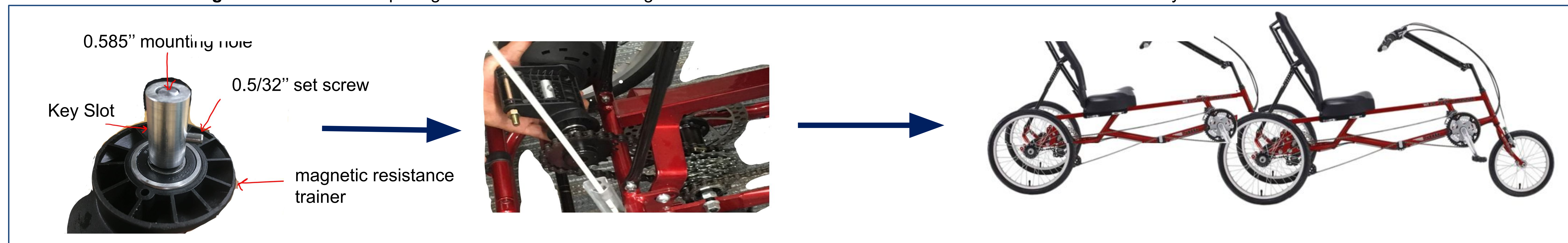
Figure 1 : Flow chart depicting the attachment of the magnetic resistance mechanism to the Sun E3 recumbent tandem tricycle.
