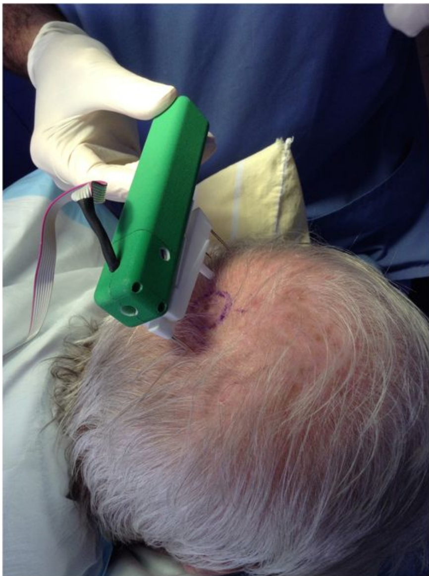
Figure 1: Skin tensiometer being used to measure scalp tension.
