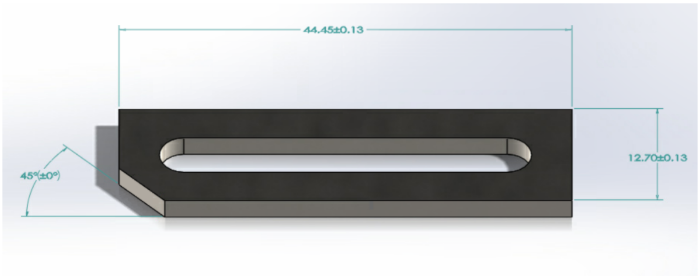
Figure 2. Model of slotted pieces. In accordance with our fabrication plan, one corner of the slotted pieces are sanded down to the width of the long piece so that they rest on the long pieces at a 45 degree angle. The angle at which the slotted pieces sit will not change how the device operates, so the team chose a 45 degree angle as it seemed the most natural.
