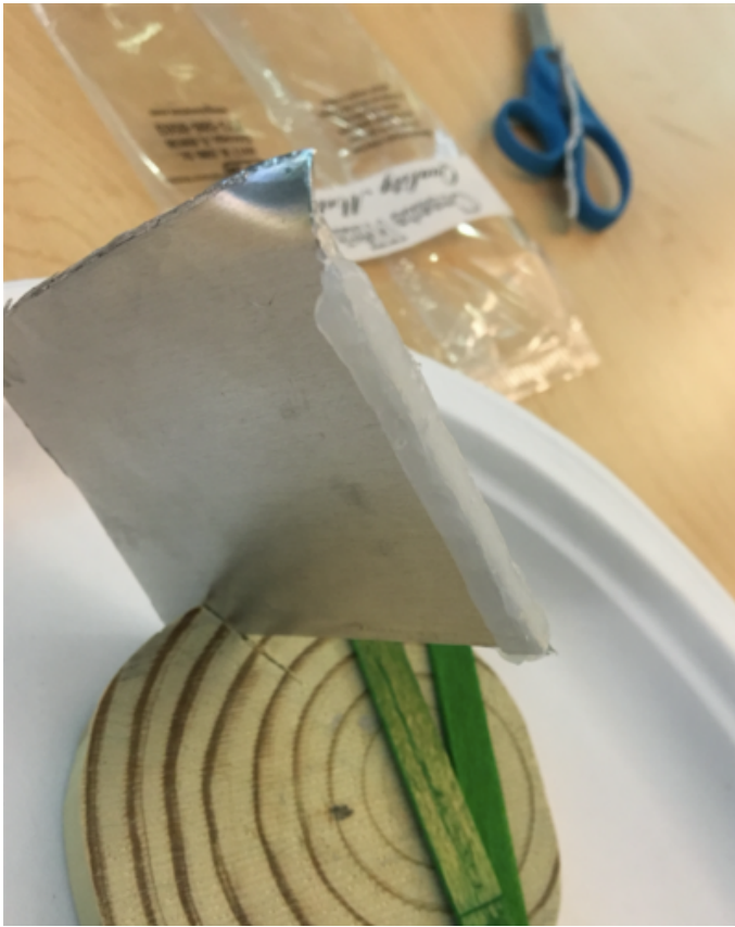
Figure 2. Testing setup that allowed the silicone to cure for 24 hours. Sample of aluminum with a large volume of silicone coating both faces and edge of the metal.
