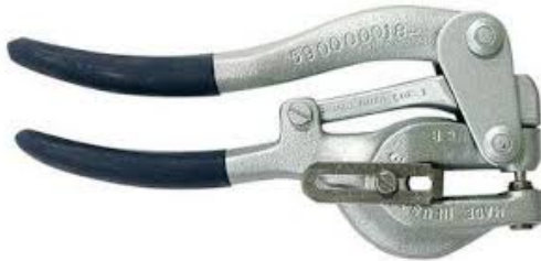
Figure 1: Whitney punch used to hollow out rectangles.
