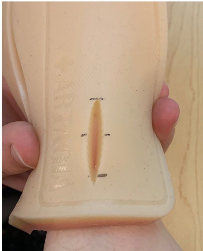
Figure 19. The laceration made on the silicone skin for testing. The skin was then draped over a forearm to cause the wound edges to splay.
