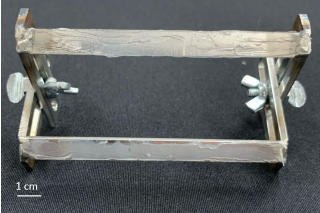
Figure 15. Bottom view of prototype displaying the thin silicone layer.
