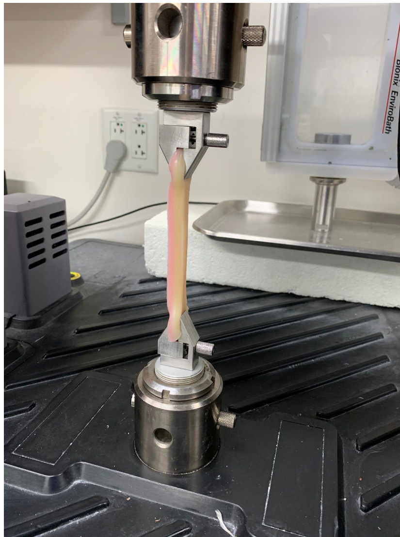
Figure 18. Image of the silicone skin strips in the MTS grips during tensile testing. The specimen was exposed to axial tension until the silicone began to slip from the grips.
