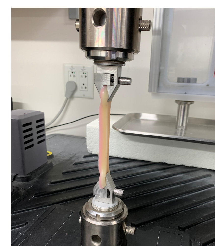
Figure 6: Silicone strip being tested in tension in the MTS machine.
