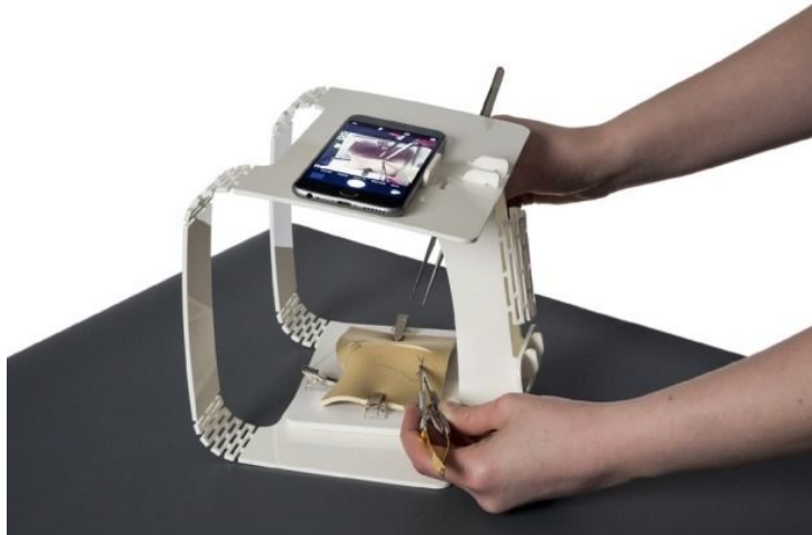
Figure 1: eoMicro simulator. The eoMicro simulator in combination with a smartphone creates a home microsurgical set-up that allows microsurgical skill improvement [3]
