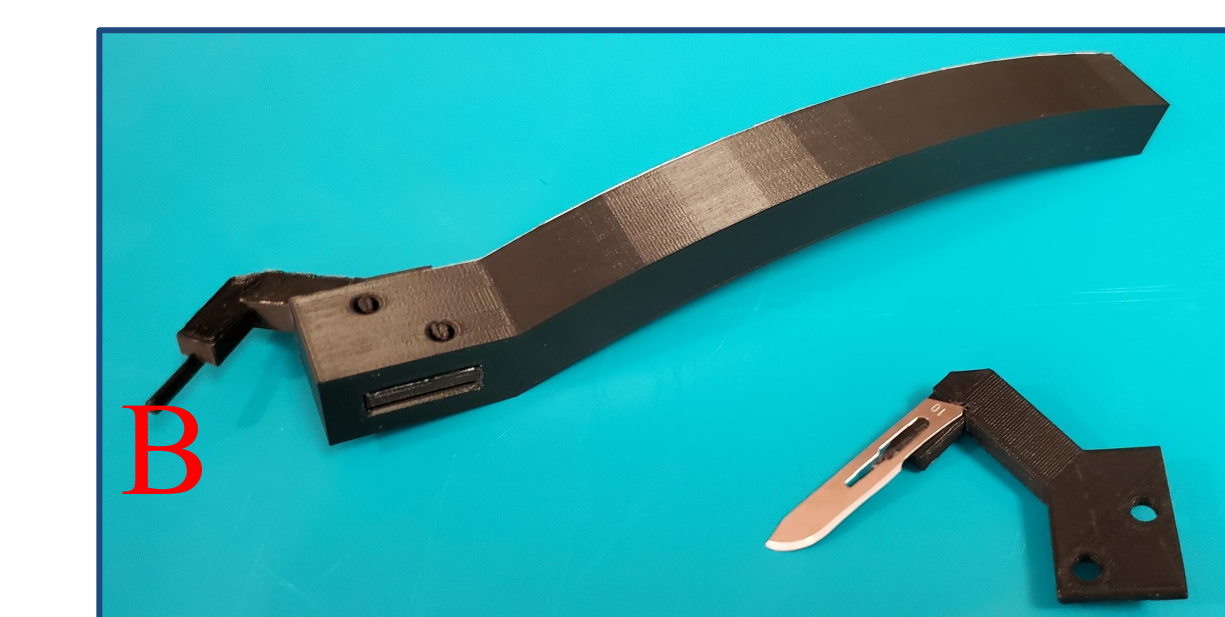
Figure 3: 3D printed prototype using High temp (A) and Tough PLA (B) arms. Both models only have the right arm in the handle due to inaccurate printing. The scalpel blade was held to the left arm, also due to a printing error
