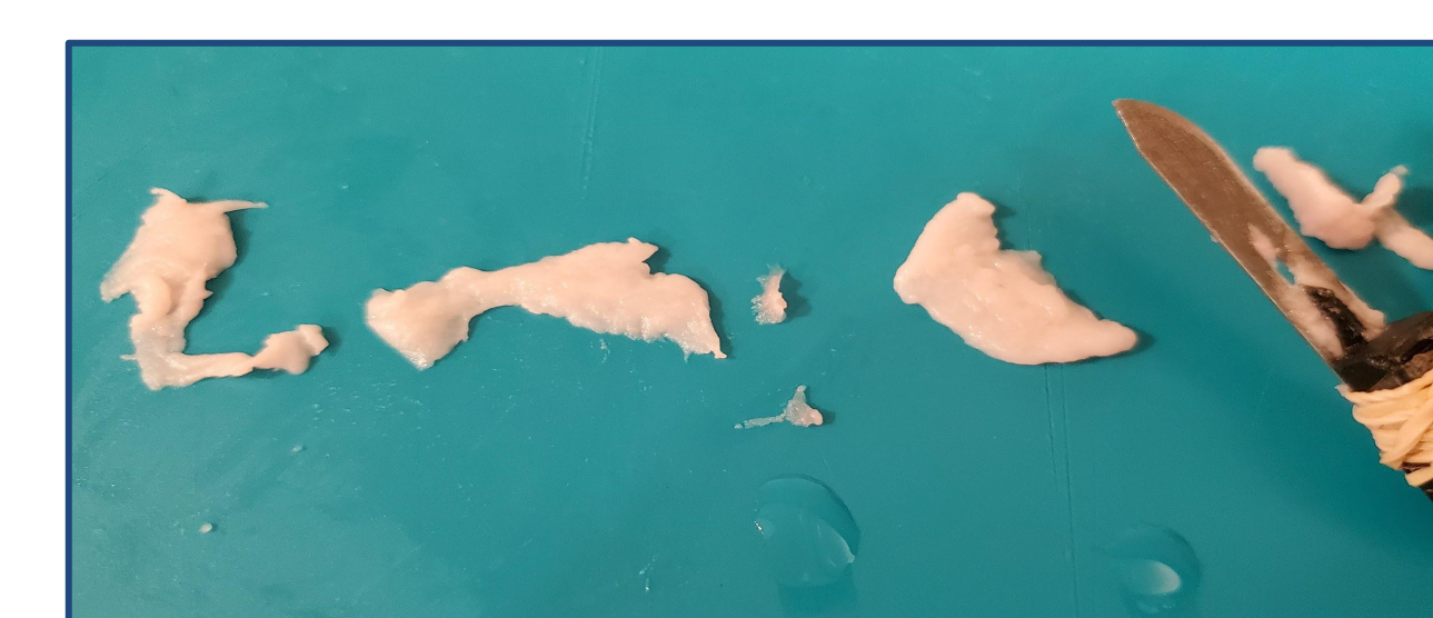
Figure 6 (above): 3D printed prototype with samples of pig tissue that were cut off. These three cuts were the only ones that were able to be successfully removed. All three lack consistency and are rough cuts due to the scalpel attachment
