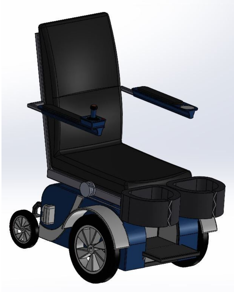
Figure 8: CAD model of the Boa System preliminary design.
