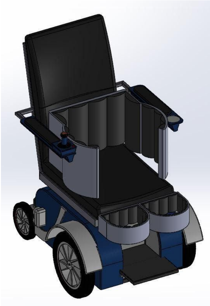
Figure 5: CAD model of the pressure cuff system preliminary design
