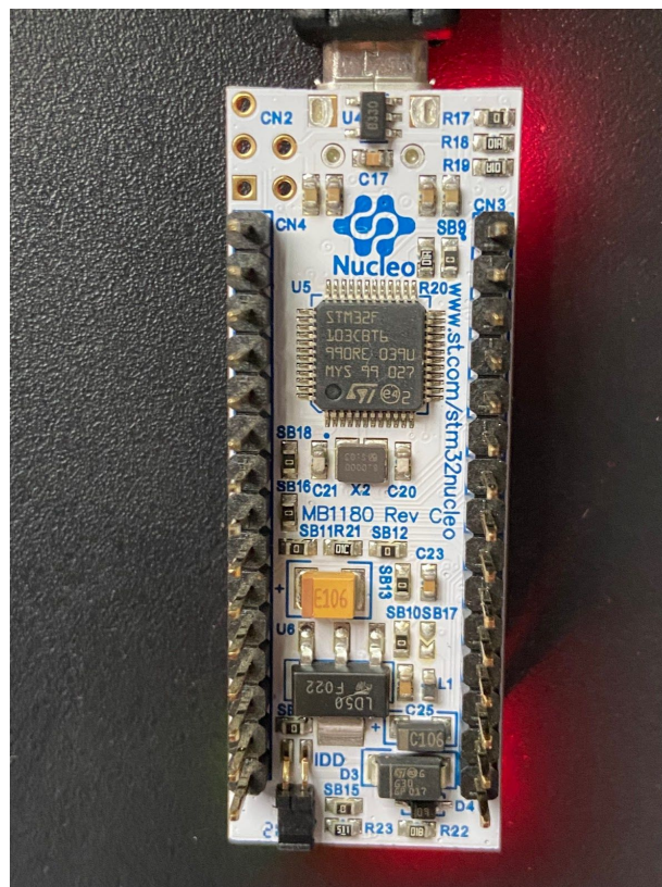
Figure 10: The Nucleo F303k8 microcontroller.
