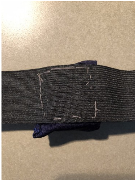
Figure 5: The sewing pattern that attached the sensor holder to the chest strap.
