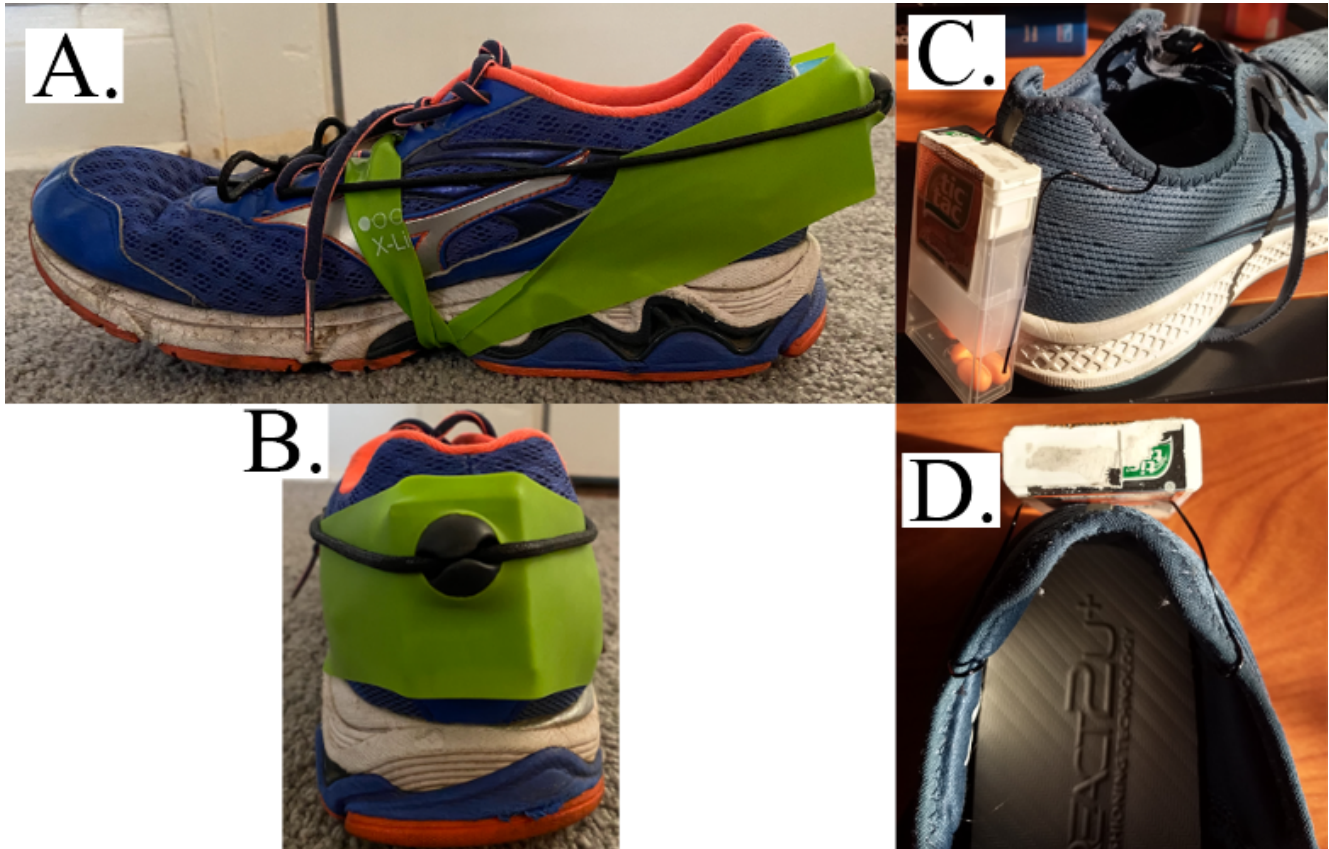
Figure 1: The graphic being used in the post. A and B correlate to the Straps design and show a side and back view. C and D correlate to the Clip design and show a 3/4 view from the back and a top-down view.
