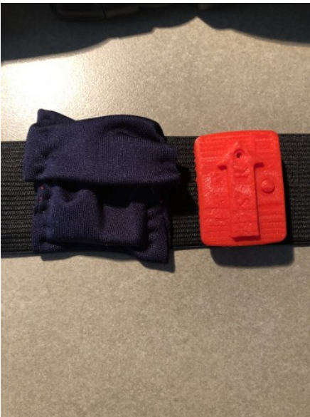
Figure 1: The sensor holder "pocket" sewn to the chest strap. 3: The pocket and sensor side-by-side.
