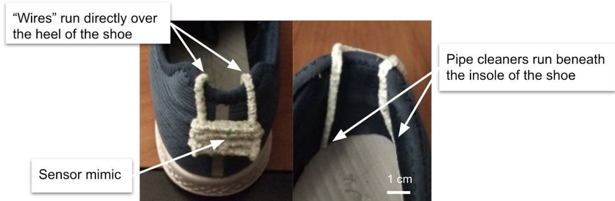
Figure 13: The proof of concept pipe cleaner model, showing the wires running directly over the heel of the shoe and beneath the insole.
