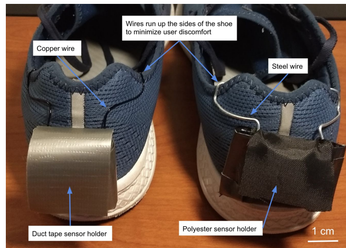
Figure 23: This image shows the final prototypes for the “Clip” model inserted as they would be during use. On the left is the copper wire model attached to the duct tape sensor holder and on the right is the steel wire model attached to the polyester sensor holder.
