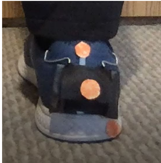
Figure 26: Current method of filming the back of the shoe with three sensor placements. In certain trials only the bottom marker was visible.
