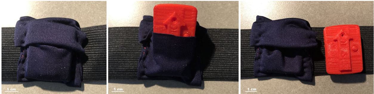
Figure 21: A progression showing how the sensor fits into the Chest holder pocket.
