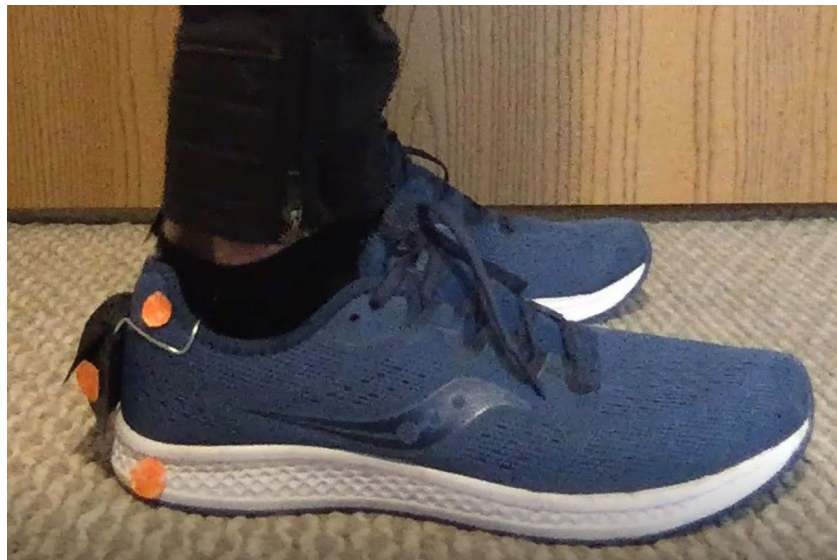
Figure 27: The placement of the three markers on the shoe. They were all too close together to currently track all three.
