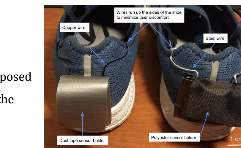
Figure 4: Both Clip designs applied to running shoes. The 18 gauge rubber-coated copper wire on the left, and the 16 gauge steel wire on the right.
