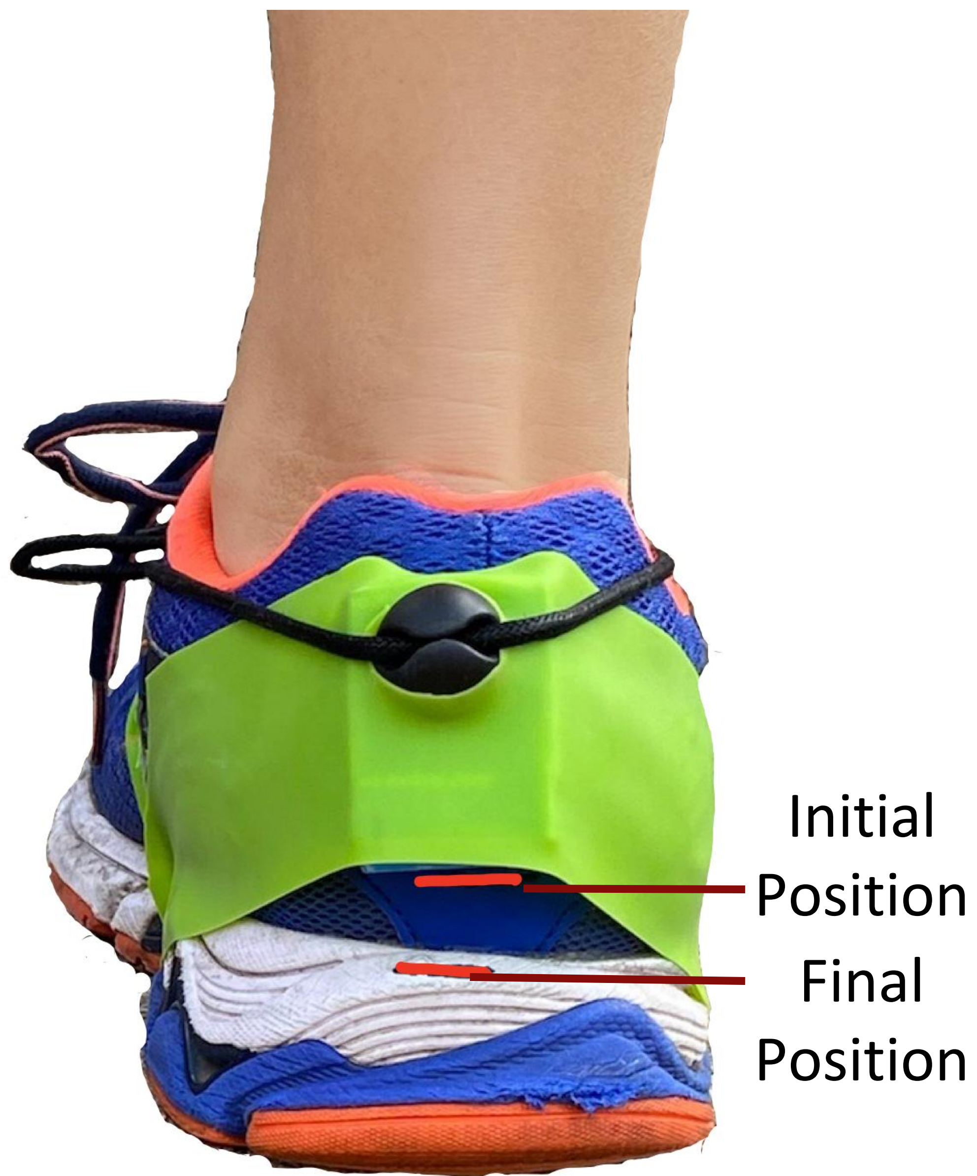
The shoe with lines indicating the positions of the sensor pre- and post-run
