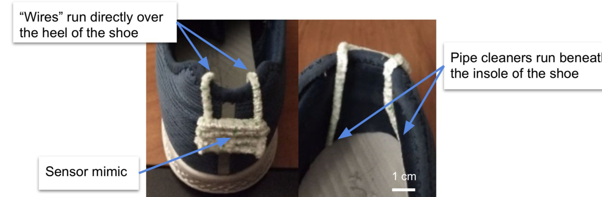
Figure 2: The first model developed to test the feasibility of the Clip design. Pipe cleaners were run directly over the heel of the shoe and under the insole.
