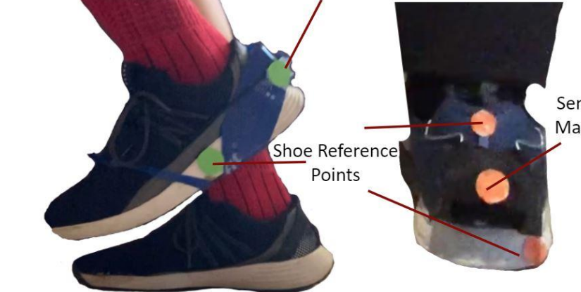
Figure 9: Screenshot of the shoe sensor holders being evaluated via motion capture
