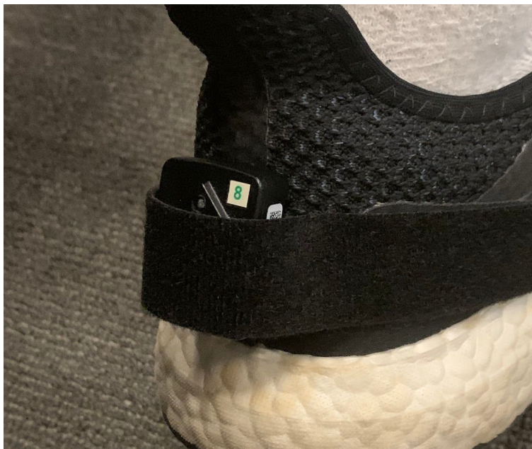
Figure 4: An image of the existing design used by Johnson Health Tech. Shown is the athletic tape that wraps around the sensor at the heel. Additional tape is used that is not depicted [5].
