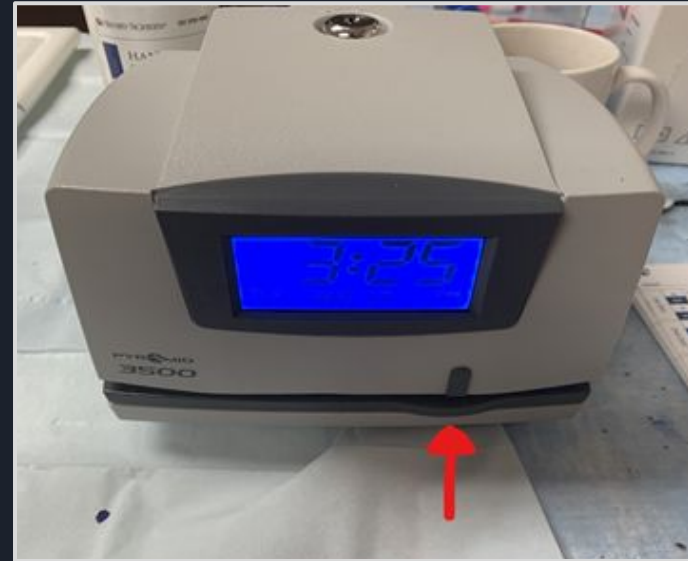
[Fig. 4] Time stamp device. Times are stamped at the red arrow
