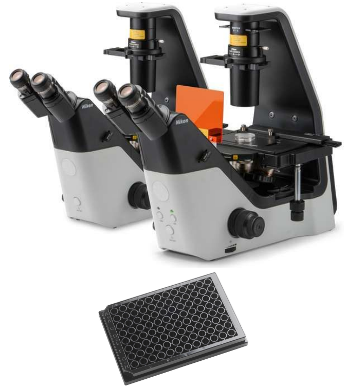
Figure 9: Nikon ECLIPSE Ts2 microscope and standard 96-well plate (opaque)
