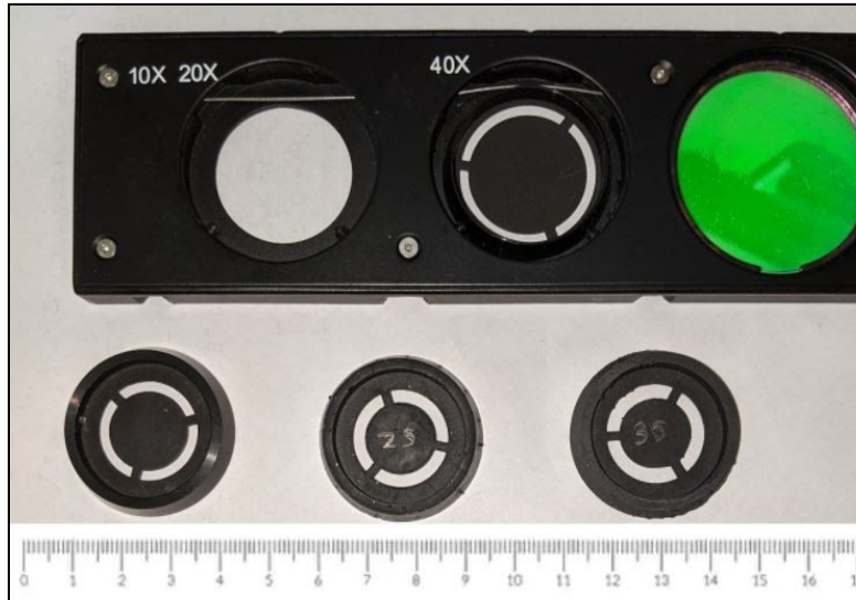
Fig. 14: The original (control) annulus (right), 25% increased annulus (middle) and 35% increase annulus (bottom). The annulus slide (top) has the far-right spot where the annuli are held in place by the thin aluminum strip that acts as a spring. Below the image is a scale bar in centimeters.
