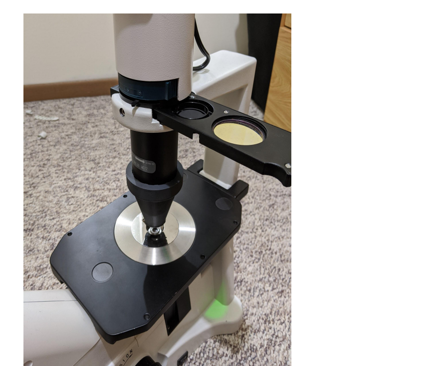
Fig. 9: The extra lens holder design is circled in green. The Design attaches to the existing microscope condenser.
