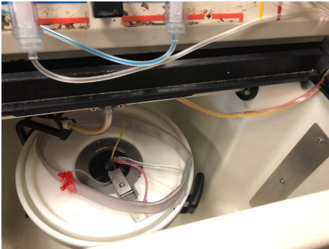
Figure 1: The centrifuge loop laid on top of the filler cap. (The diameter is much too small and the four blood component tubing sets are attached to different parts of the loop. This presents a problem since the current cap has all of the component tubings laying side by side.)
