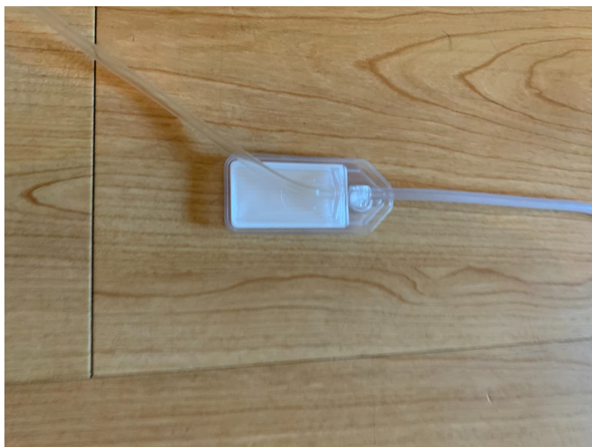
Figure 1: The Original Bubble Trap ferrule, darker component is the nut)
