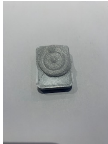
Figure 4: The bottom housing block with foam membrane substitute
