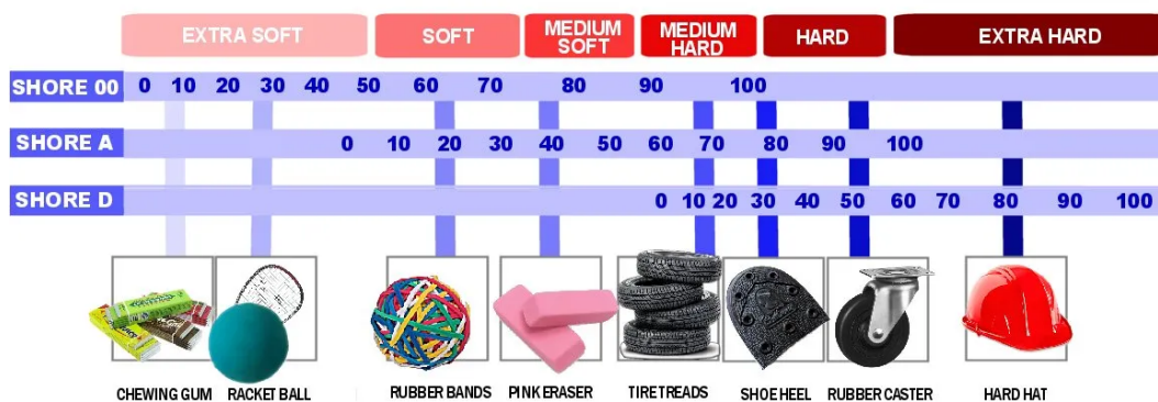
Figure 1: Shore Hardness Scale [1]
