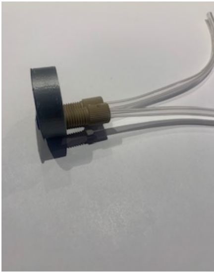
Figure 3: The nuts twisted on to the top housing block
