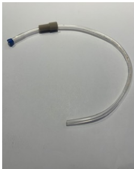
Figure 2: Tubing with flangeless fitting attached (Blue component is
