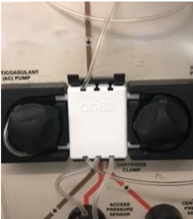
Figure 2: Partially loaded tubing set with too much slack around the pumps
