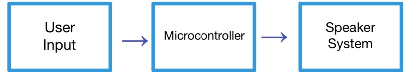
Block Diagram for Dial Controlled Speaker Design
