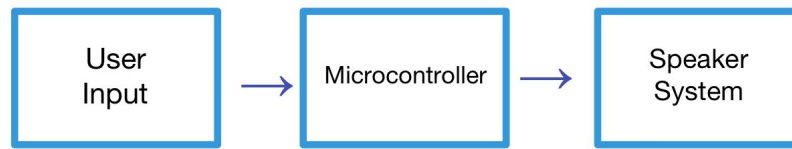
Figure 7: Dial-controlled speaker block diagram. This system is a simple three step process where a dial would be directly connected to the microcontroller which would then emit signals to turn the speaker system on and off.
