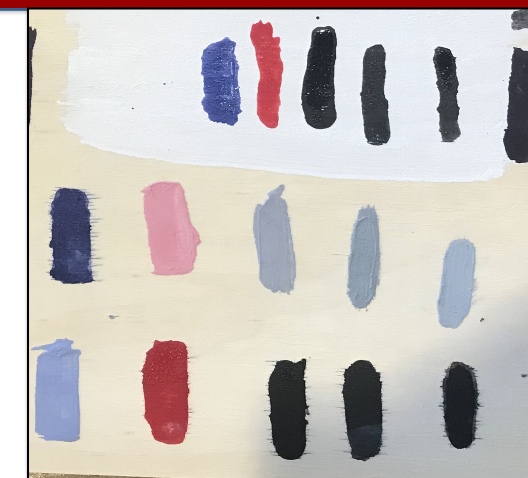
Figure 2 - Image of swatches of TLC pigments on wood, resulting in very weak color change
