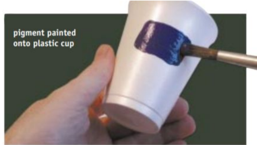
Figure 14 - Thermochromic powder used as paint [13]
