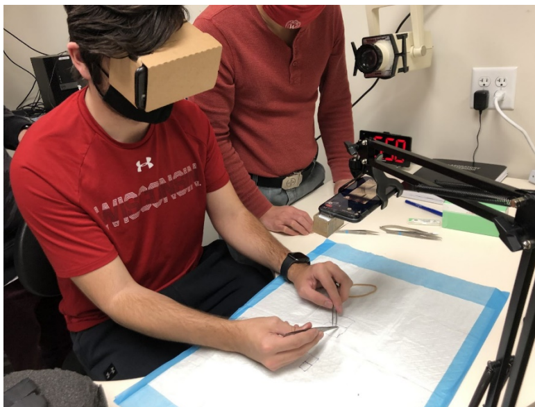
Figure 17: Testing on depth of perception by a team member. With Google Cardboard on, the member is trying to move sutures with a tweezer via the video streamlined from a smartphone with the attachment.
