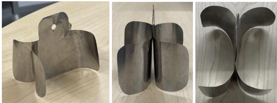
Figure 13a, 13b, and 13c: Enlarged Prototype. From left to right a view of the front, side, and top are shown. Take note of the curved corners and included hole on the top tab.
