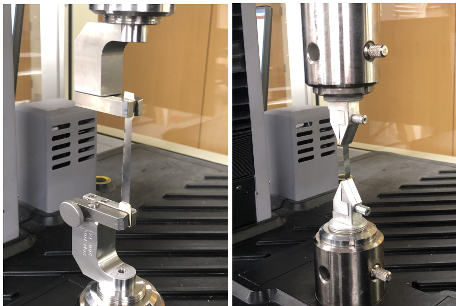
Figure 20a and 20b: Two different fixtures being used during MTS testing. The fixture on the left seemed to lead to much later slippage and was the fixture primarily used.
