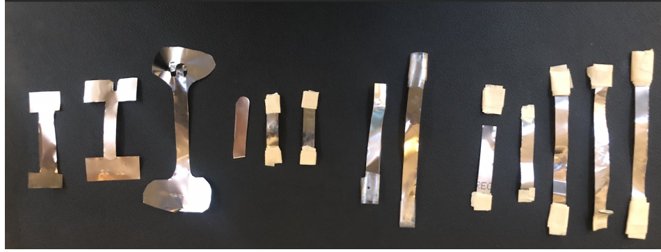
Figure 19: Samples that were used in the MTS Machine. A variety of methods above are shown that were used in attempts to avoid slippage such as the tape and dog bone cutouts.
