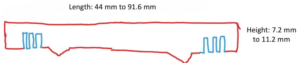
Figure 4: Handcuff Design Side View. Length, measured left to right, should be in the range of 44 mm to 91.6 mm. Height, measured top to bottom excluding “spikes”, should be in the range of 7.2 mm to 11.2 mm. Slot fittings, in
