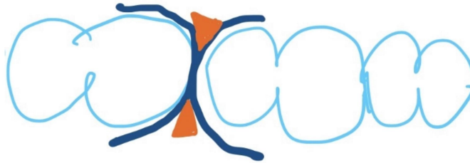
Figure 7: Butterfly Design installed. This hand drawn image shows how the butterfly band (dark blue) would sit between teeth (light blue) and be held in place by two wedges (orange).
