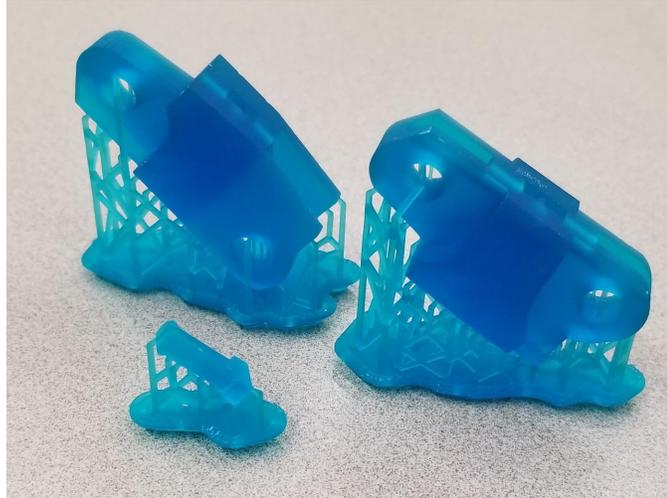
*Figure 8a. Formlabs resin prints are seen above with the complex support structure still attached. This structure is easily separated to provide a high quality finish. These prints were the first to include the intricate tunnels running through the top and bottom of the part.*
