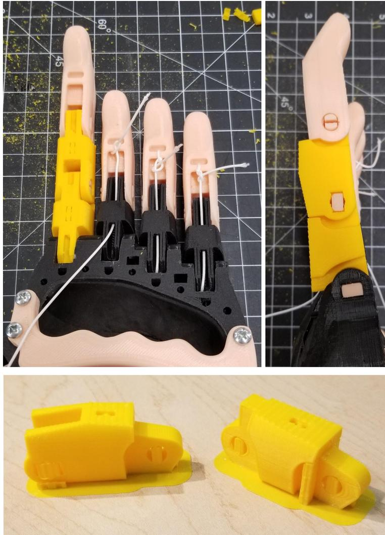
*Figure 9. The prints above were intended to be the first set of final prototype prints, however, an error in printing led to the incorrect material being used and the prints were considered a failure.*
