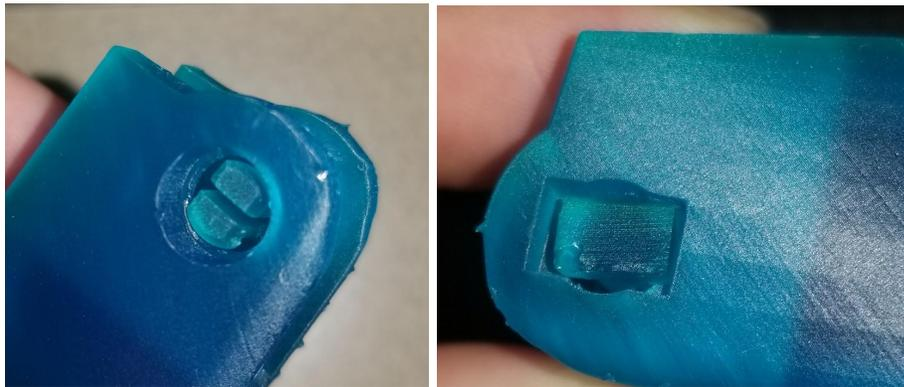
*Figure 8b. The pin inside of the phalanx component is significantly smaller in diameter than expected, a key lesson moving forward in parts scaling. Note the very smooth, high quality finish of the part. This finish is achieved, at an increased price.*
