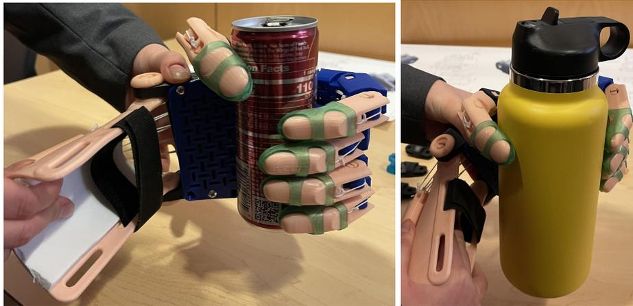
Figure 14: Seen above is the arrangement of components during the qualitative testing. A Redbull can and Hydroflask are seen being gripped here.
