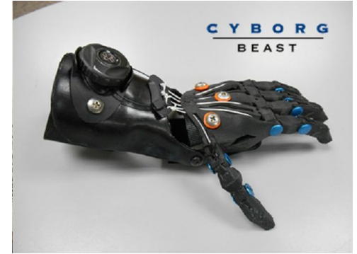
Figure 2: The Cyborg Beast 3D printed hand is one of the competitors for accessible 3D printed prosthetics [1]
