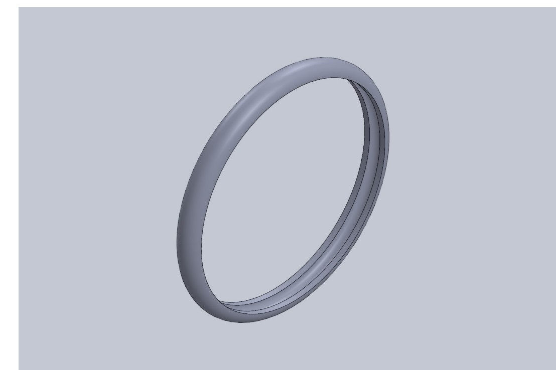
Figure 2. Final Design Guidewire Hoop. Outer Radius: 11 cm. Inner Radius: 10 cm.
