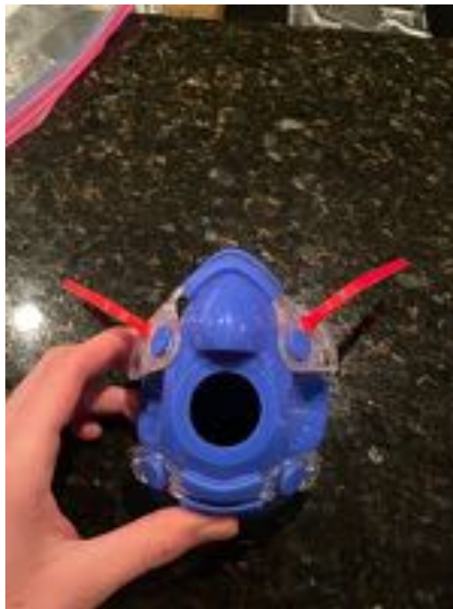
A2AB047C-CAF3-40CD-9C31-67A61819C040.jpg(552.9 KB) - download Printed Pieces Attached to Structural Brace on Mask
