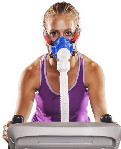
Figure 1: Subject demonstrating the use of the CardioCoach VO2 max testing.
