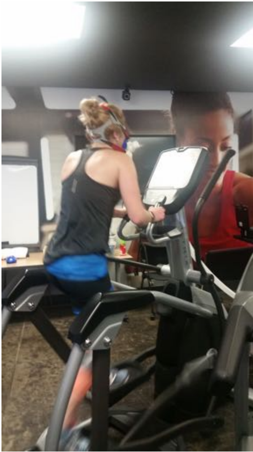
Figure 5: Subject using the existing VO2 masks with straps visible
