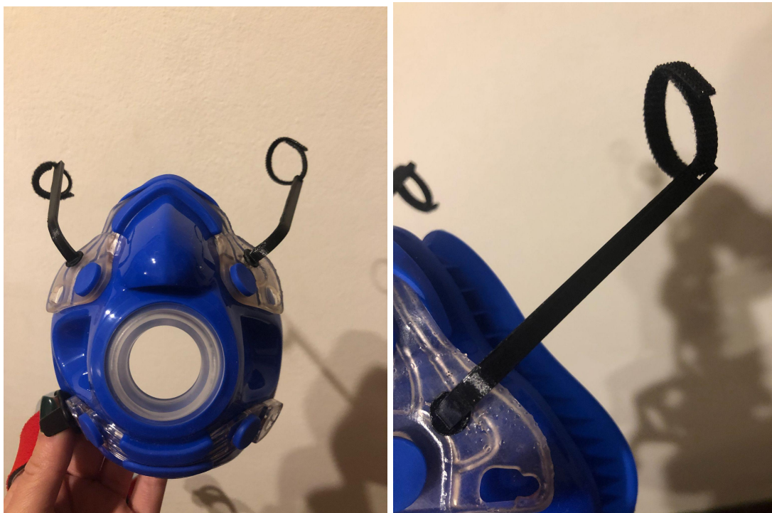
Figure 19-20: The proposed final design. The extension pieces connect to the newly printed structural brace piece and have slits that Velcro straps can insert into and wrap around the legs of the user's glasses to provide stability and comfort.
