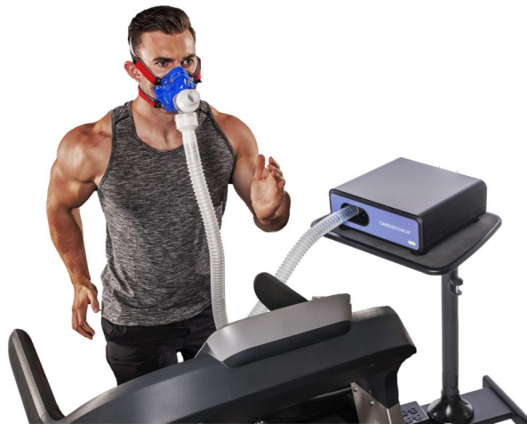
Figure 4: VO 2 max testing set-up.
