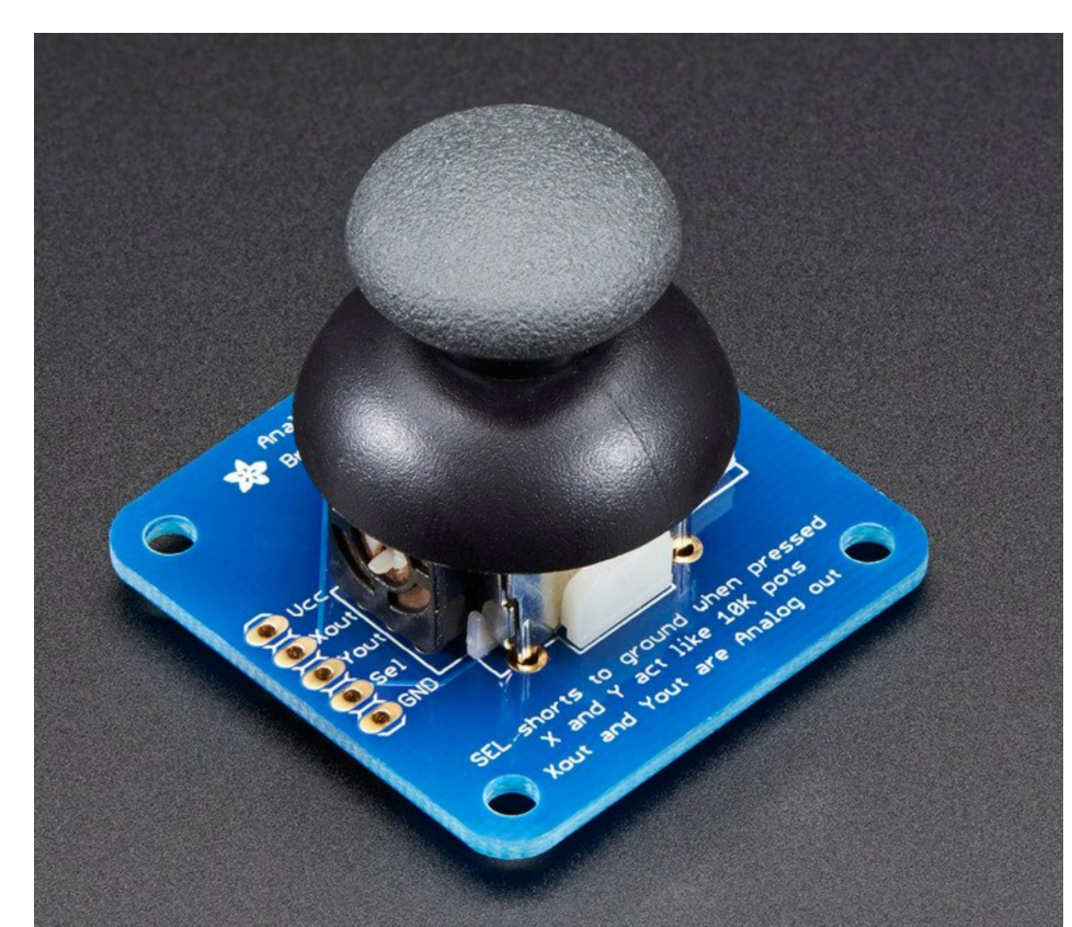
Figure 13. The thumb joystick used in the circuit.
