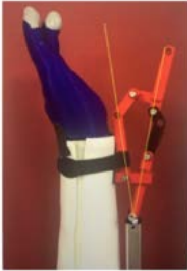
Figure 22: Example measurement of ImageJ analysis. Pictured is angle of full flexion, not example calculation. ImageJ measures an angle of 18.35 degrees.
