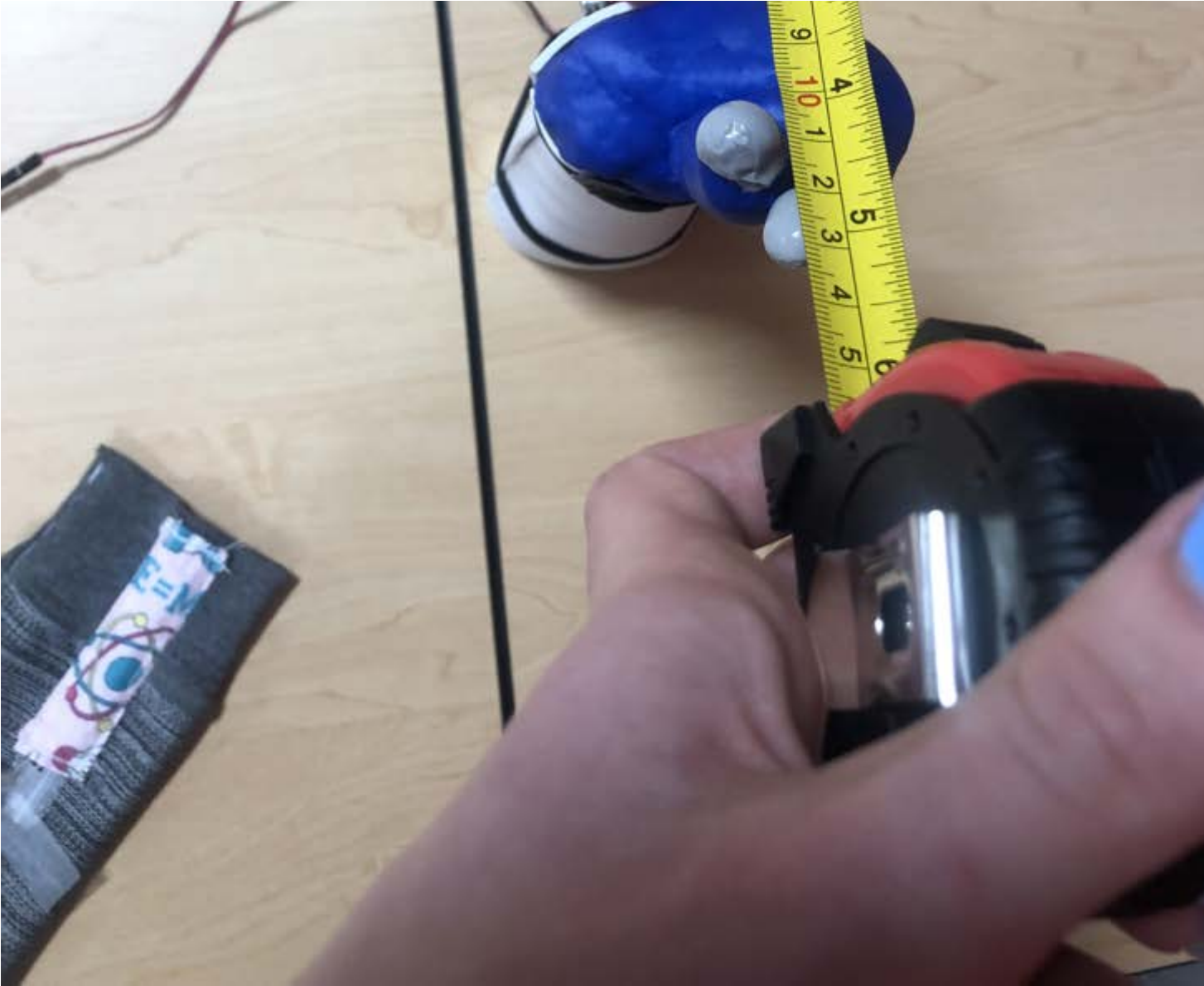
Figure 24: Measuring the range of motion of the prosthetic thumb.
