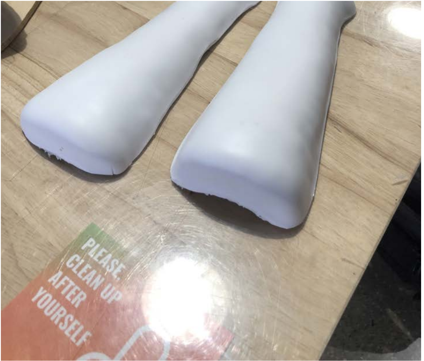
Figure X: The two cuff pieces after initially being cut out.
