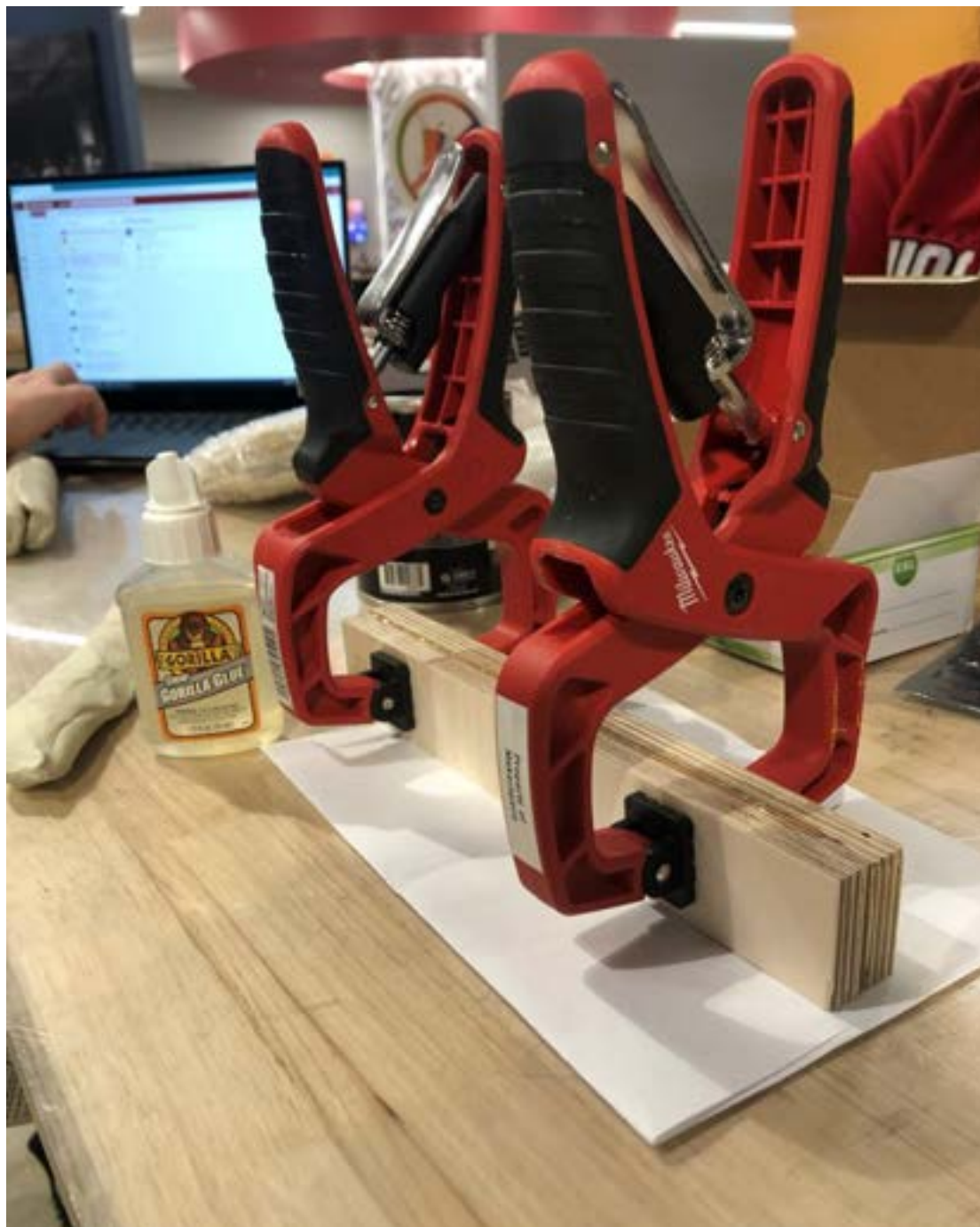
Figure 17: Base material of plywood being glued so that clay can be formed around it.
