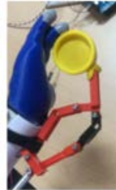
Figure 23: The prosthetic thumb successfully holding a small container.
