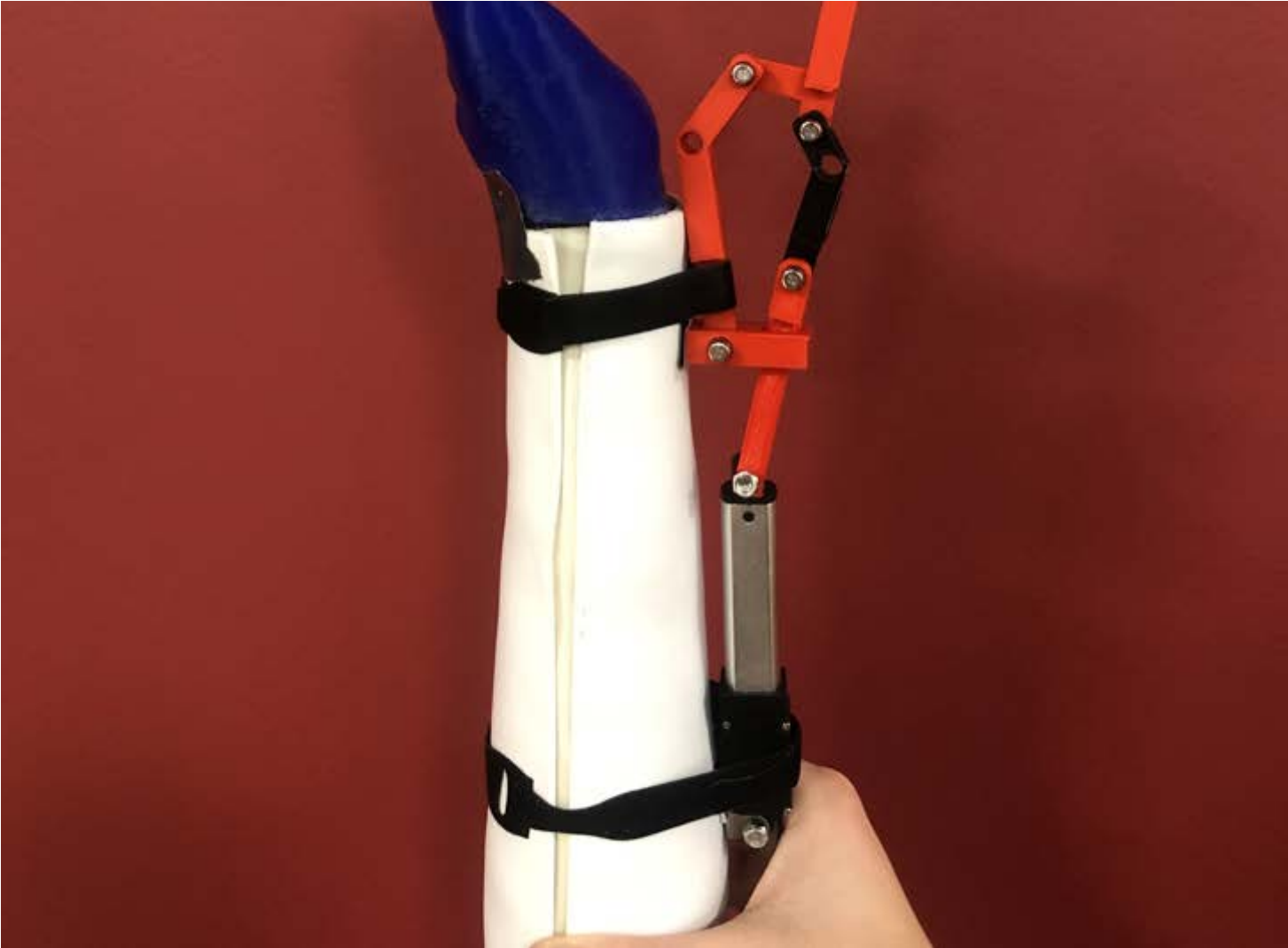
Figure 23: Final working prototype of the prosthetic thumb.
