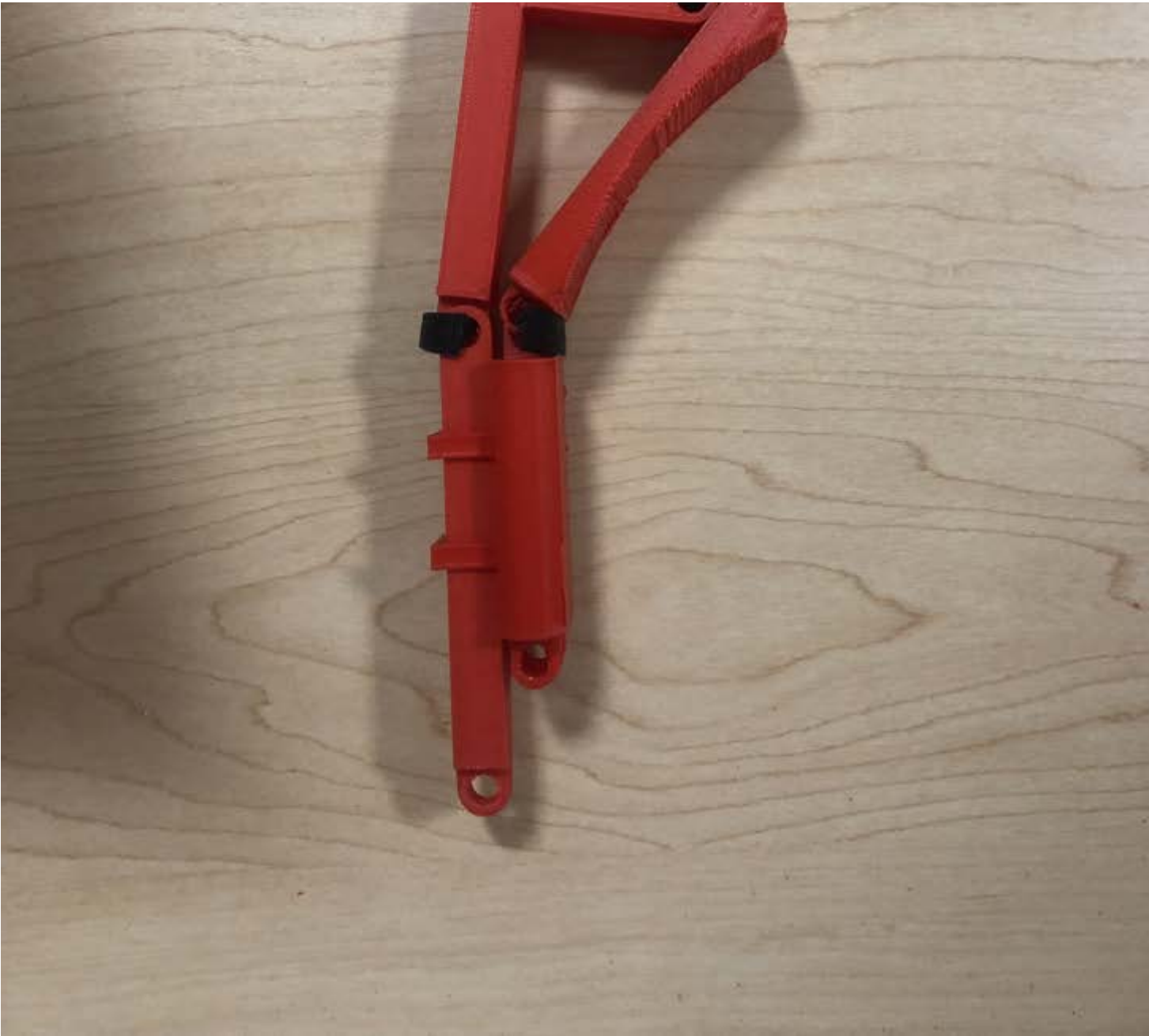
Figure 25: 3D Printed Design of my design using velcro clasps because the pins did not fit.
