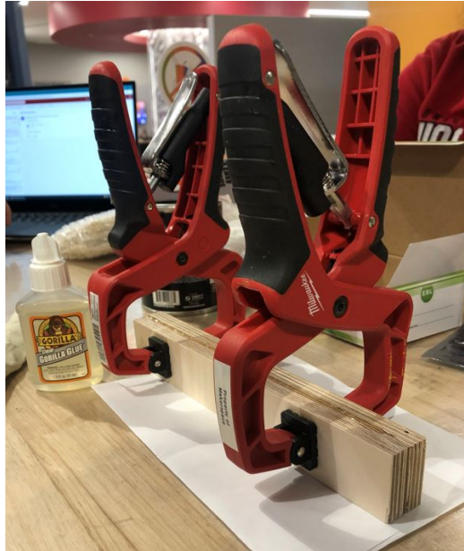
Figure 16: Two pieces of plywood being glued together to act as the core material for the model forearm. The strong core provided a backbone for the clay to be molded onto.
