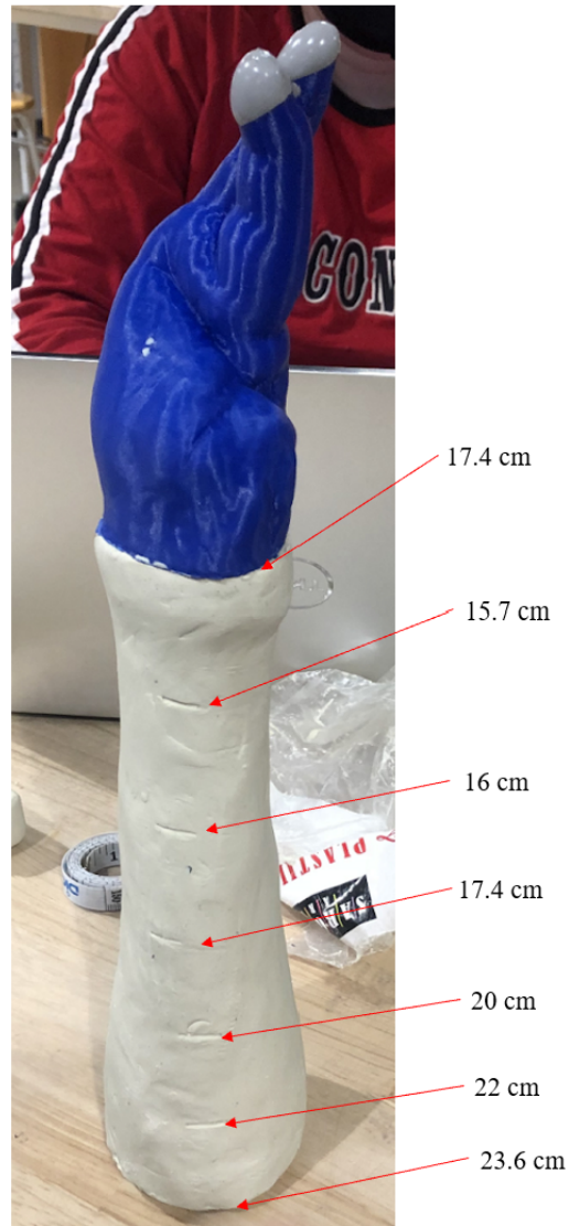
Figure 17: The completed forearm model with a 3D model of the patient's hand set on top. Measurements depict the cross sectional circumference at various points along the arm
