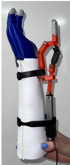
Figure 20: Picture of the final design.
