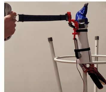
Figure 21: Example of Force Testing with a Crane Scale. The handheld force sensor was held still while the prosthetic thumb flexed.
