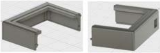
Figure 2: CAD diagram showing the fabrications of the stage enclosure in two components
