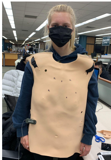
Figure 9 (left). Final Prototype. Final Prototype being worn with pulse monitor and adjustable clips. Figure 10 (right). Close-up of electronics. Bluetooth Speakers integrated on the inside.
