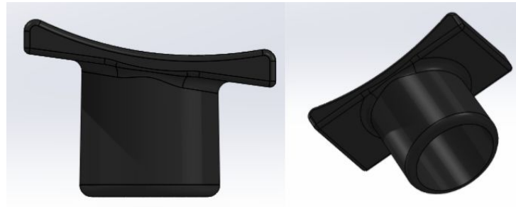
Figure 8: CAD model of the polymer tips used with the adapted Weitlaner design
