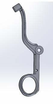
File: 'LockMechMale\_v2.SLDPRT' (Male component of the locking mechanism)
