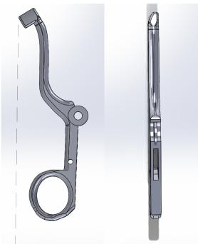
All fits together well with the 4.5 mm pin well. Still need to update the pins to screws and find a locking mechanism geometry that works
