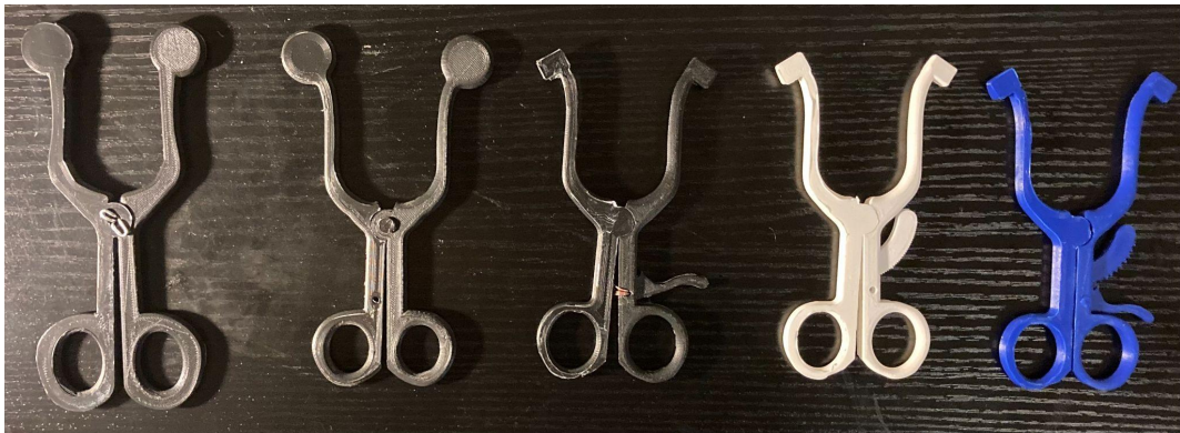
Figure 14: Five iterations of the device from the earliest (far left) to the most recent (far right). Improvements involved changes to the locking mechanism, distal end geometry, and ergonomics of the handle.
