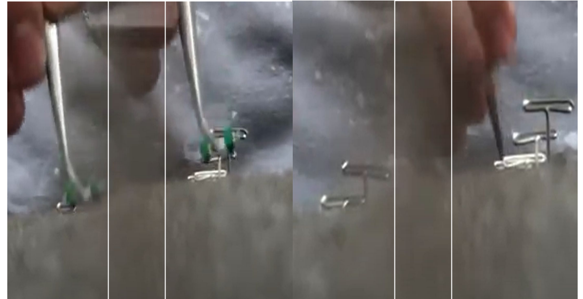
Figure 7: Visual of workspace through lens with rectangles outlining the slight blind spot in the middle of the image
