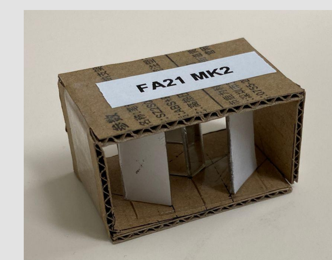
Figure 2: Early proof-of-concept prototype design utilizing a double-mirror array fabricated from cardboard.
