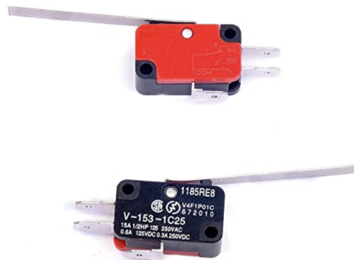
Figure 20. Limit Switch. A limit switch [16] will inform the Arduino about whether the adaptive side of the machine is in use. Based on this feedback, the program will rotate the console as needed.
