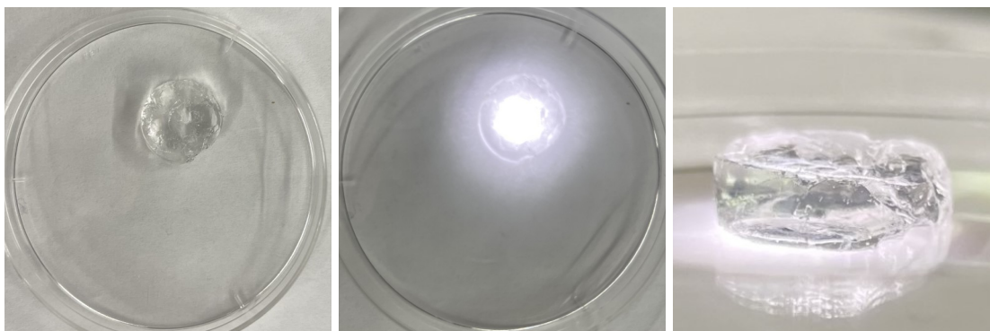
Figure 1: Gel before shining light (left), and gel during translucency testing viewed from the top (middle) and from the side (right)
