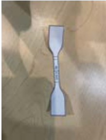
Figure 1: Sample template of dog bone shape
