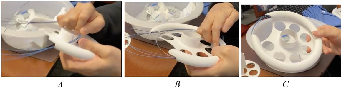
**Figure 4.** Insertion of guidewire (GW) into wheel.
