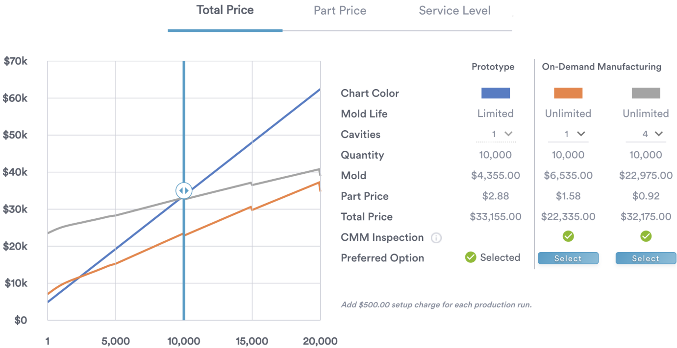
Figure 6: Quote for 10,000 top pieces to be injection molded. Note the cost of the mold for just the top part ($4,355.00)
