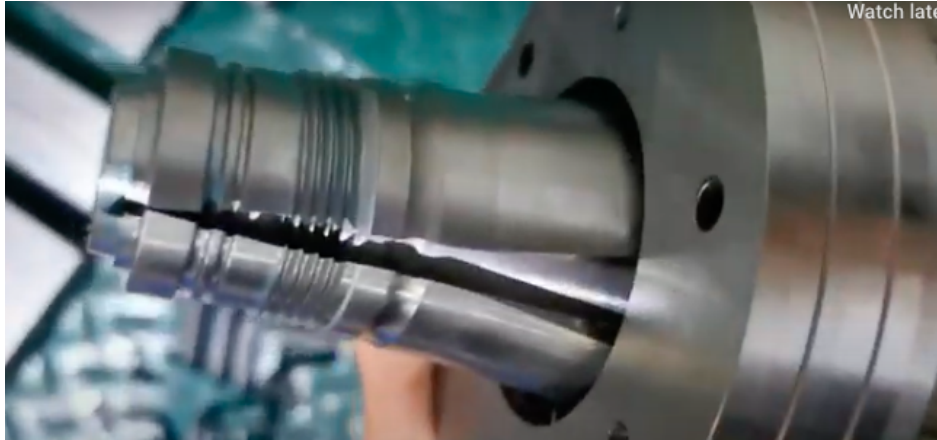
Collapsed to remove and eject part (Smaller outer diameter of the part)
