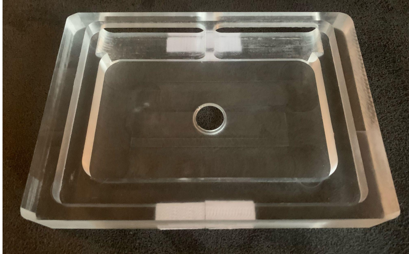
Figure 10: An image of the underside of the stage top platform that was created using a mill.
