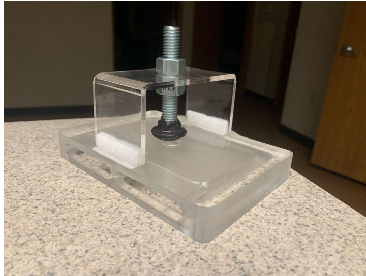
Figure 11: An image of the final prototype. The clamping mechanism is attached via velcro and then the bolt is put through the hole.
