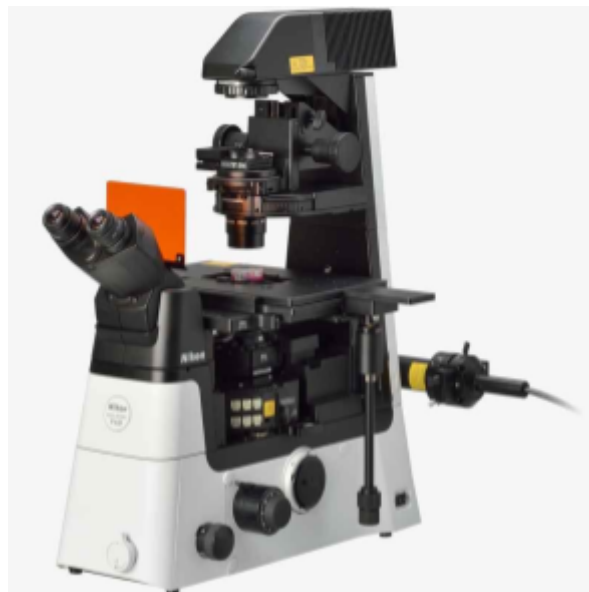
Figure 1: Nikon TI-U Fluorescent Microscope [1]
