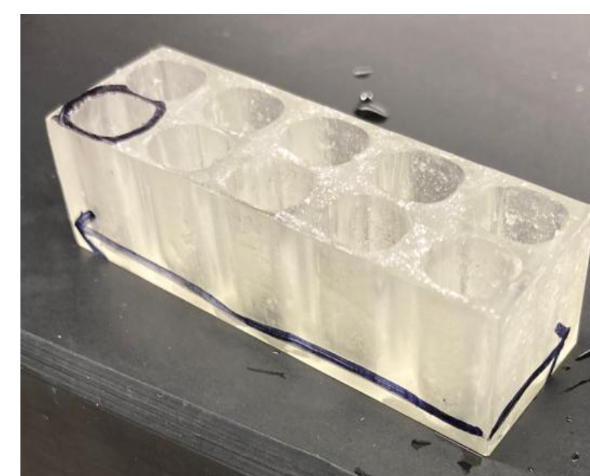
Figure 3.3: Mouse sizing array resin, chosen circled. Dimensions: height 9mm, width 7.8mm and 45° width of 7.8mm.
