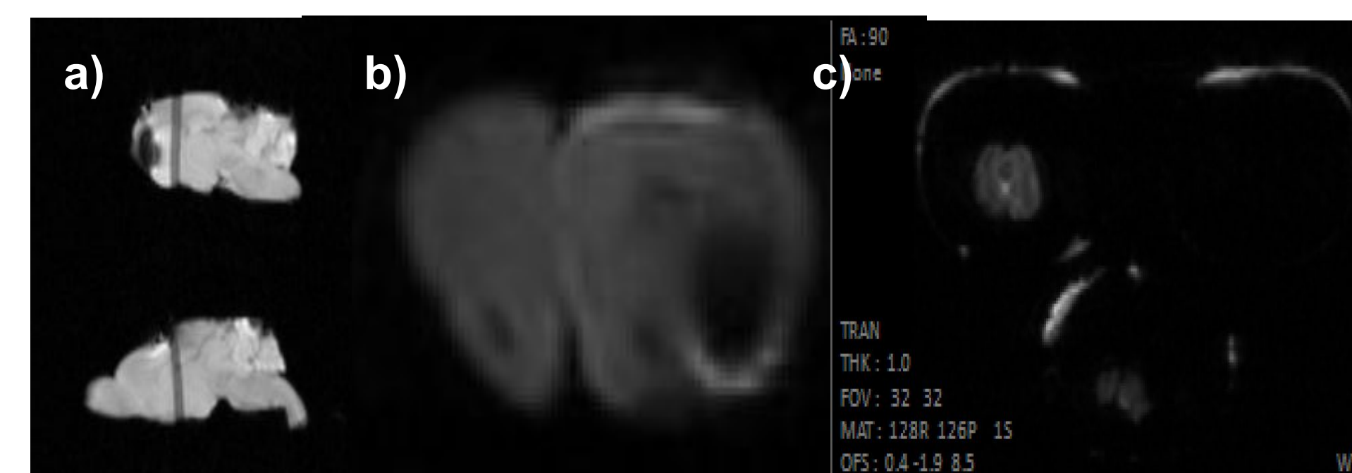
Figure 3.6: Final scans. a) brains tilted down approx 15° on side view. b) air bubbles caused black circle. c) water trapped under o-rings from water tests appear on MRI scan.
