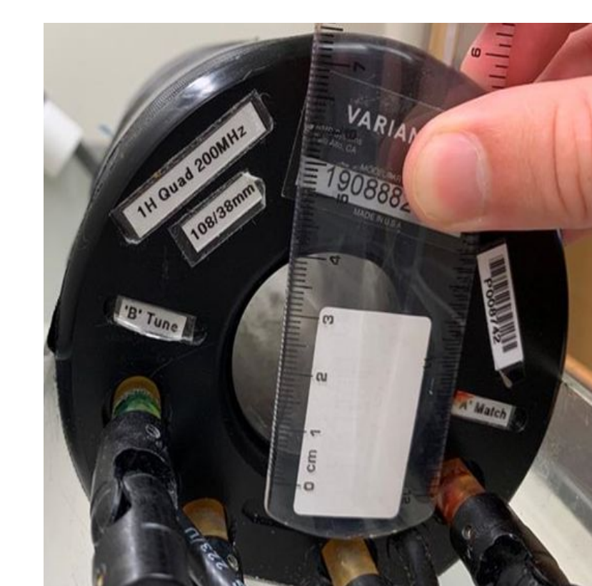
Figure 2.1: Coil inserted into MRI with 37.6mm diameter bore
