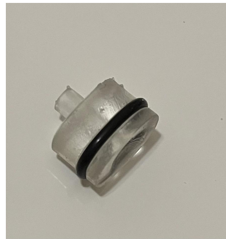
Figure 34. Rat brain capsule cap in FormLabs clear resin with rubber o-ring.
