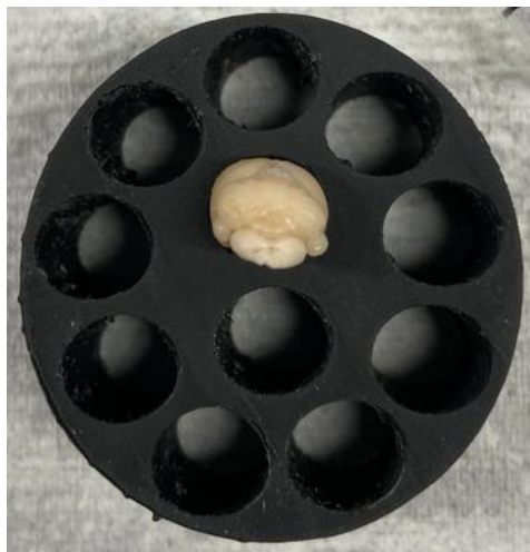
Figure 21. Mouse brain not fitting in initial mouse capsule prototype in FormLabs black.
