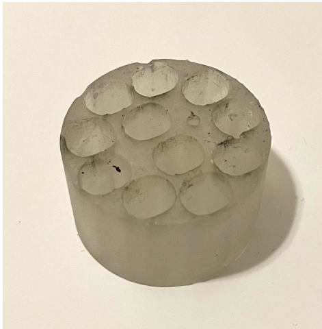
Figure 28. FormLabs Clear mice brain capsule with updated hole dimensions and 2.5mm diameter watermark hole.
