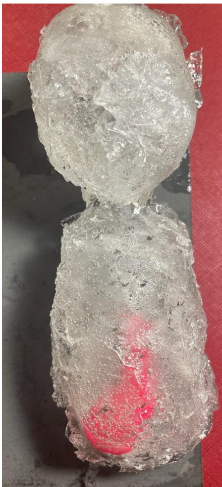
Figure 4: Final prototype made out of Sylgard 184 with intubation tubing and balloon mechanism
