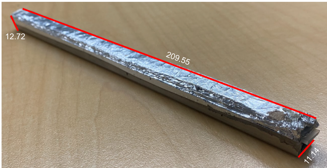
Figure 15: A trimetric view of one of the side dampers with one section of the foil exterior removed. Dimensions are in mm.
